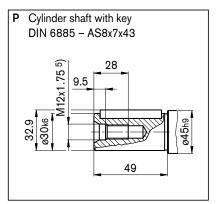
Before finalizing your design, request a binding installation drawing. Dimensions in mm.
