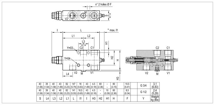
\* The adjusting screw can be completely unscrewed. Do not exceed the indicated protrusion range of the adjusted screw.
